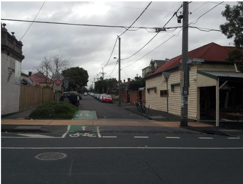
Example of partial road closure (no entry, bicycle excepted) with raised threshold at entry to local street, Brunswick, Victoria.
