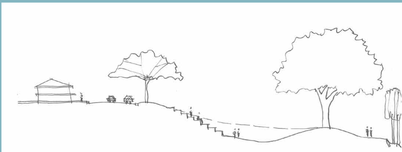
Orleigh Park retrofit: terraces and fig mounds created to allow a lower park area which can spread floodwaters during peak events
